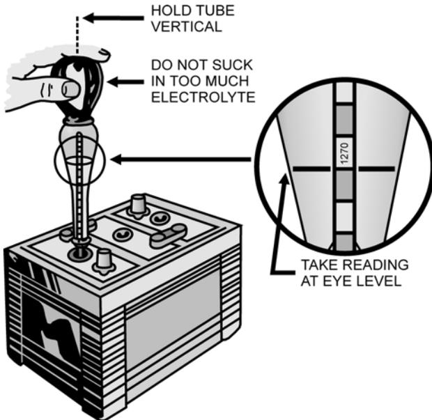
Testing Specific Gravity of a Battery
