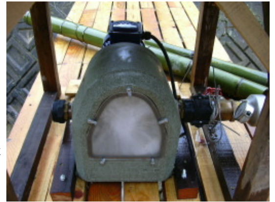
generator built-in turbine unit
