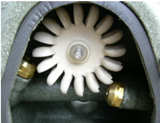
Small pelton generates small energy at 300watts at maximum, but works for 24 hours.
