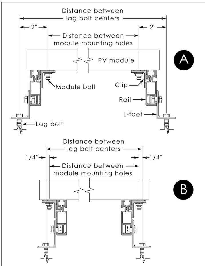
**Figure 2. Clip Arrangements A and B**
