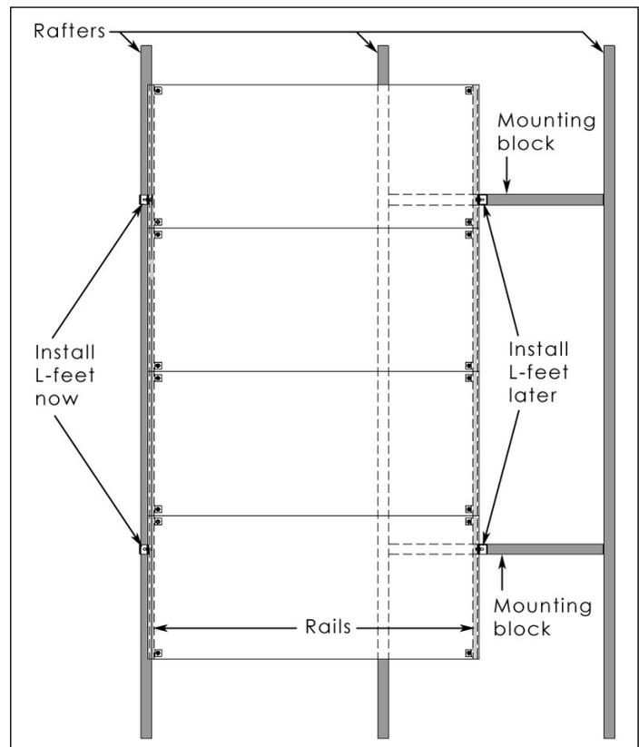
**Figure 4. Rails laid out parallel to the rafters.**
