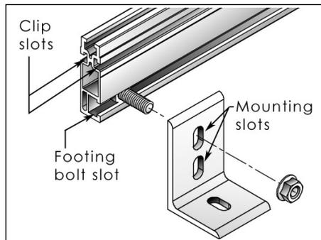
**Figure 5. Leg-to-rail attachment**
