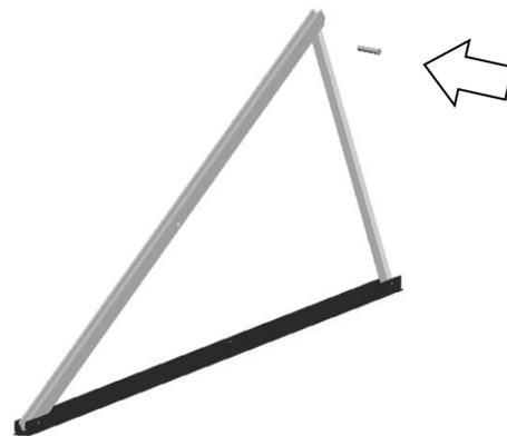
5.1.3 Fix the tubes with U Bracket to the base support by using hex head bolts M10\*65, Spring Washer, Flat Washer and Hex nuts M10.
