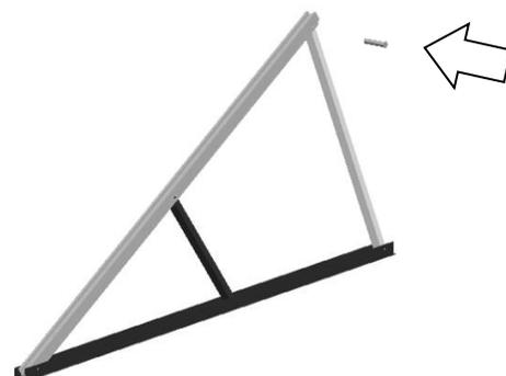
5.1.3 Repeat the step above for each support that you need to install. Fix the support Tripod to the purlin following the planning guide.
