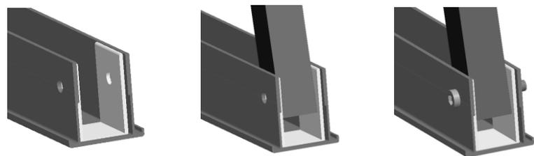
5.1.2 Unfold the middle tubes in the upper support (if you use double Tripod), fix them to the base support by using hex head bolts M10\*65 and Spring Washer, Flat Washer and Hex nuts M10.
