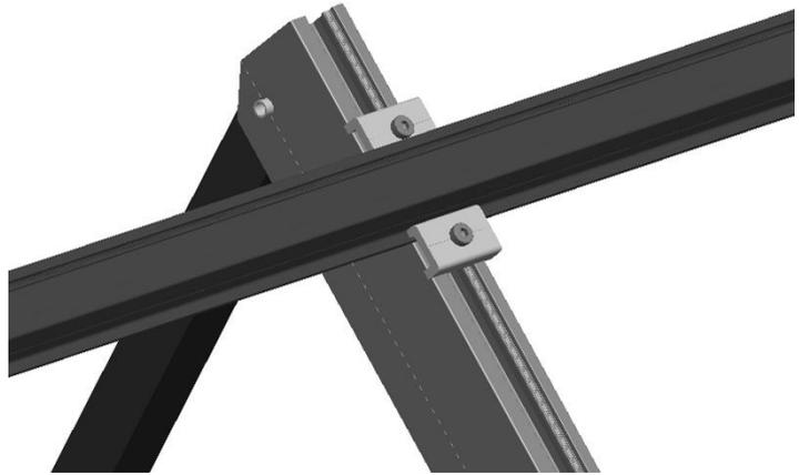
5.3.2 If the rail is not long enough, please connect the rails by using the splice for T rail 50 using 2 tek screws on each side.
