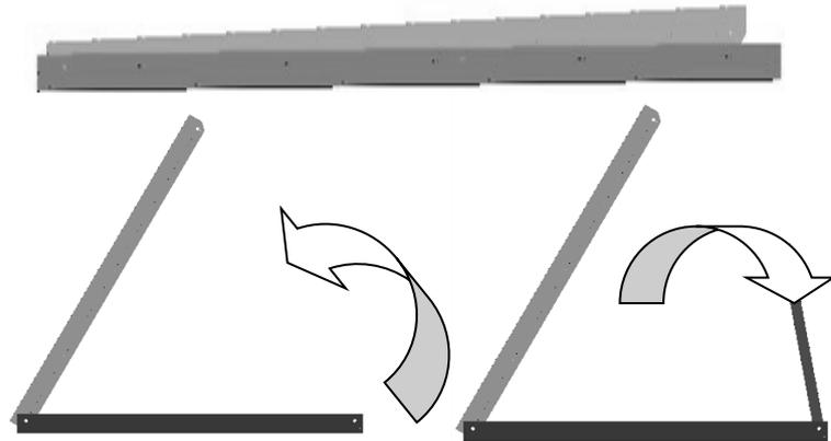
5.1.2 Fix the back tubes to the upper support by using hex head bolts M10\*65, Spring Washer, Flat Washer and Hex nuts M10.
