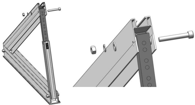
5.1.2 Tighten the screws through the leg strut to go along with the positioning groove on the leg tube, in order to achieve accurate positioning purposes.
