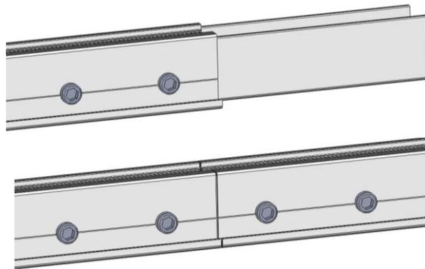
5.3.3 Fix all the rails on to the upper support as the step above.
