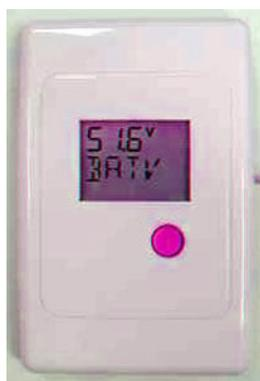
The PLM remote monitor is a device which allows remote user access to a PL series charge controller. It shows exactly the same information as the PL screen and the PLM button behaves in exactly the same way as the button on the PL. This means you can use the PLM for everything you would normally do at the PL itself, only in a more convenient or second location. You can access all the same information and adjust all the same settings as you can on the PL itself.
