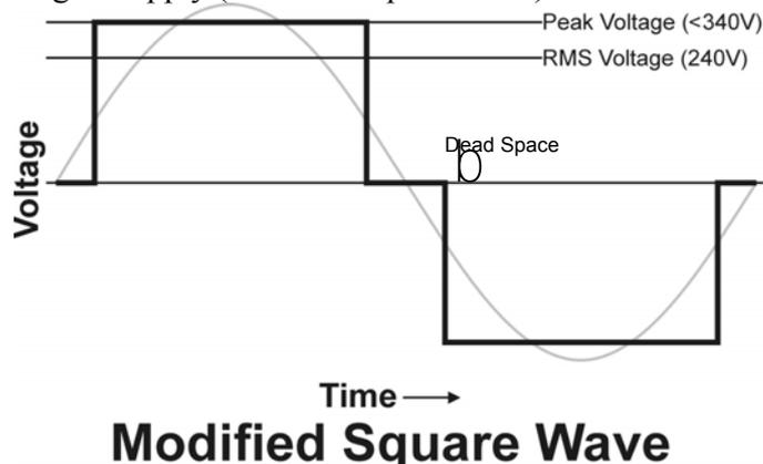
"Modified square wave" or "stepped wave" is where the force of the electricity is varied by having an intermediate step in between changing direction. This wave form approximates more closely to a sine wave than does the "square wave".
