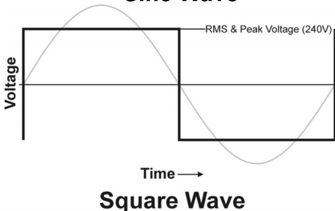
Some (particularly the older style) solid state inverters produce "square wave", "modified square wave" or "stepped wave" electricity. "Square wave" is the term used when the electricity has a constant force, such as it has with DC but switches direction more or less instantly at the same kind of frequency as the normal grid supply (at 50 times per second).
