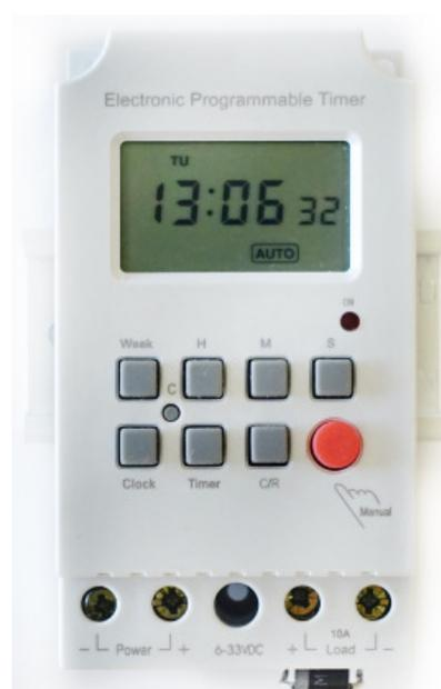
**Connect timer to a 12 or 24 volt DC supply with correct polarity.**
