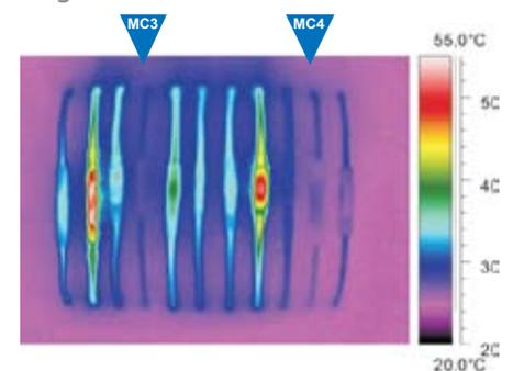
A temperature increase test by the TÜV Rheinland with PV plug connectors from various manufacturers shows significant differences in the rise in temperature and the excellent results of MC-PV connectors.
