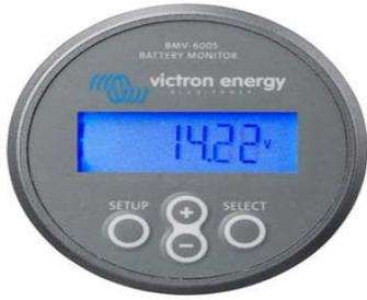
The essential function of the battery monitor is to calculate ampere-hours consumed and the state of charge of a battery SOC. Ampere-hours consumed is calculated by comparing the current flowing in or out of the battery. Section 3.4, p10 of the BMV manual has descriptions of all the available functions of the BMV.
