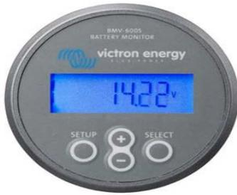
The essential function of the battery monitor is to calculate ampere-hours consumed and the state of charge of a battery SOC. Ampere-hours consumed is calculated by comparing the current flowing in or out of the battery.
